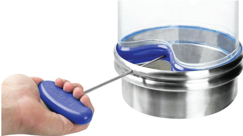
Once a BFM® TR connector is fitted, it is virtually impossible to remove it manually. It is, however, straightforward to remove using a TR Release Tool, which is simply inserted into a 6mm hole in the side of both the upper and lower spigots.
