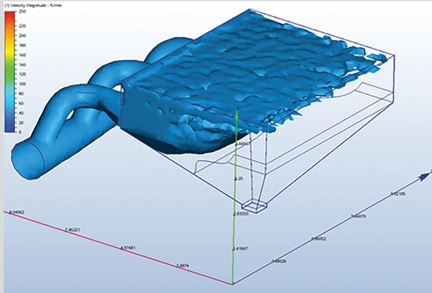
Computer Fluid Dynamics (CFD) analysis is used to locate problems in the air stream and indicates where improvements can be made. Our expert team utilizes CFD analysis to verify hood, duct work, and filter design for energy efficient and robust systems.
