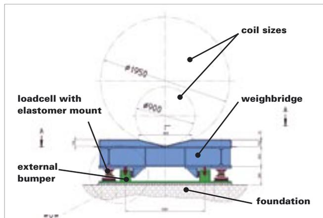
Fig. 14: Basic structure of a legal-for-trade coil scale 35t
