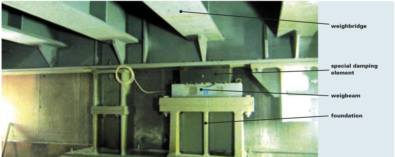
**Fig. 11: Scrap platform scale 130t with Schenck Process Weighbeams DWB (Courtesy: ThyssenKrupp Nirosta)**
