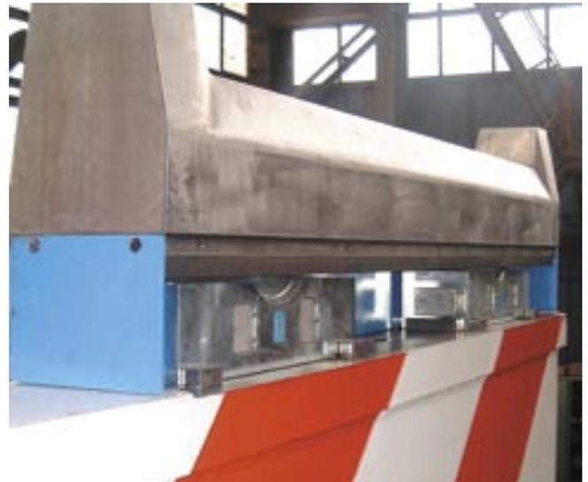
Fig. 2: Weighing unit of a 350t ladle turret (Courtesy: Siemens VAI)
