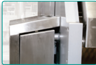
Angled surfaces for drainage
