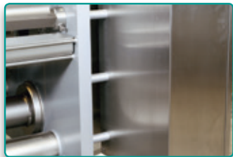
Holes eliminated where possible
