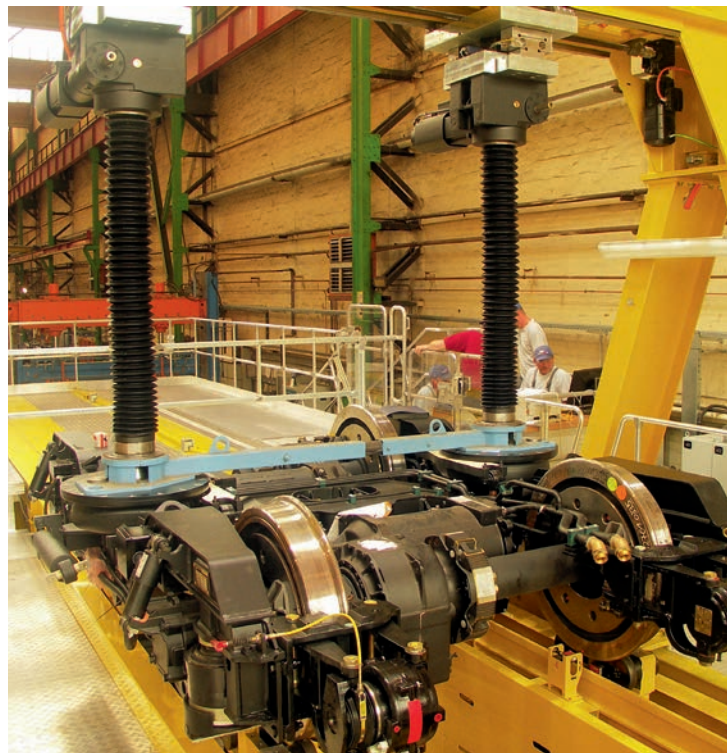
Testing with air suspension via adapter crossbeams
