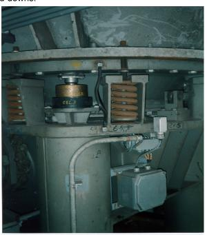
For standard bin weighers the conventional solution - using Loadcells RTN and Compact Mounts VKN - still remains the most economical solution in future. Nevertheless for systems with special installation conditions, like the here discussed supporting point of the top -hopper silo of a blast furnace, such as
