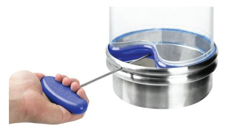
Once a BFM® TR connector is fitted, it is virtually impossible to remove it manually. It is, however, straightforward to remove using a TR Release Tool, which is simply inserted into a 6mm hole in the side of both the upper and lower spigots.
