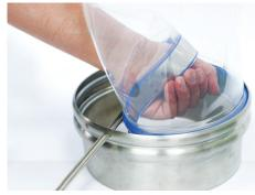
Hold the seal of the connector and remove from the spigot.
