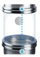
Snap into the second spigot, ensuring that the welded seam of the connector is straight and that points A and B are directly in line.
