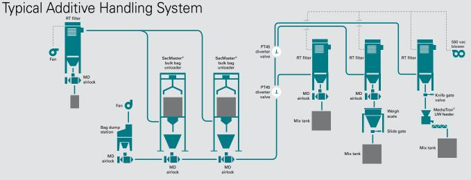
Lithium Hydroxide/Lithium Carbonate Storage & Transfer Systems
