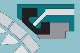
The seal automatically inflates only when the dome is fully closed.
