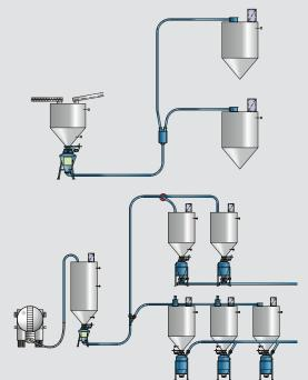
The range of pumps for dense phase conveying are designed for different applications according to the material and the distances the material is to be conveyed. The range of dense phase pumps are:
