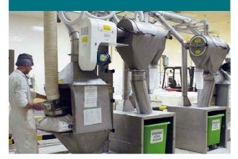
Sifted material is then discharged directly into the lidded wheeled tubs within collection booth directly below the Sifter outlet. Any agglomerates etc therefore separated and not processed.
