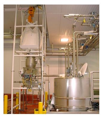
With the cracker meal/cake flour supply feeder in the proper position, the operator starts the batching process using the touch screen of an Allen Bradley VersaView® 1500 M HMI station. Weight signals from IP68 rated stainless steel load cells positioned under each leg of the system; control the run cycle of the feeder and the flow of cracker meal or cake flour to the selected mix tank.
