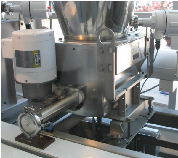
A vibratory feeder accurately dispenses an ingredient into a chocolate base bar's recessed cavity.
