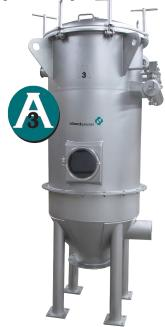
the Schenck Process HRT 3-A filter becomes an excellent product receiver. Product enters the filter and is discharged from the bottom through an airlock. Centrifugal force separates the product from the airstream and gently discharges it.
