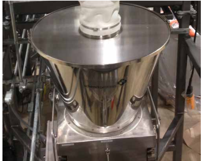
Refilling a continuous gravimetric feeder takes careful timing and measuring of materials.
