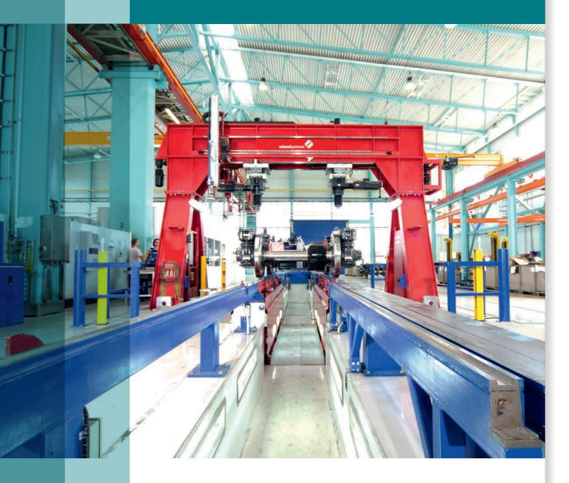
Quiet, comfortable and low-wear rolling trains are the result of intensive development work. Schenck Process helps vehicle manufacturers and maintenance workshops to take reliable measurements in bogie checks and corner load measurements.
