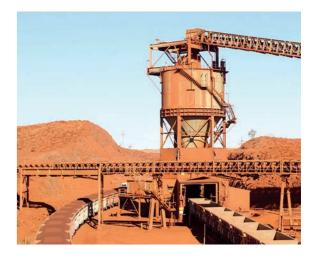
MULTIRAIL® Dynamic Train Scales for Loading can weigh wagons immediately before and after loading thanks to precision measuring technology. This allows maximum use to be made of wagon capacity without the wagon weight exceeding the permitted track load.
