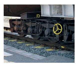
MULTIRAIL® Dynamic Train Scales for Hot Metal is for precise determination of hot metal output for blast furnace operations.
