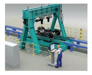
MULTIRAIL® Bogie Test Bench is part of a new generation of bogie test rigs fit for the future. One prominent feature is the fully electro-mechanical design with spindle technology which ensures extremely efficient work practices and high levels of precision.
