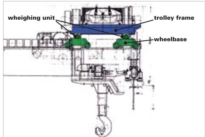
**Fig. 5: Basic structure of weighing in the area of the wheelbase (Courtesy: Arcelor Gent (SIDMAR))**
