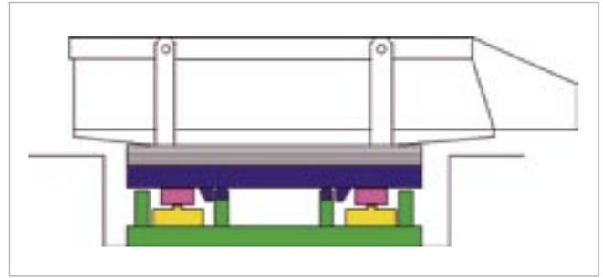
**Fig. 10: Basic structure of a platform scale for scrap loading**
