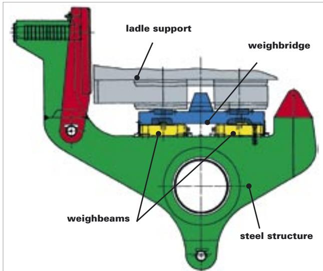
Fig. 1: Basic structure of a ladle turret scale
