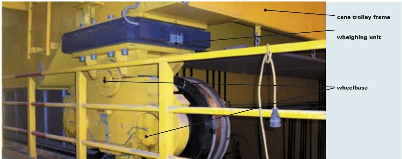
**Fig. 6: Weighing unit of a 400t ladle transport crane (Courtesy: Siemens VAI)**
