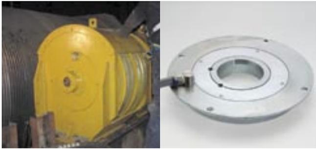
**Fig. 8: New upper sheave block 350t with pre-assembled DRA-sensors (Courtesy: Ternium Sidor), Fig. 9: Schenck Process Radial Force Sensor DRA**
