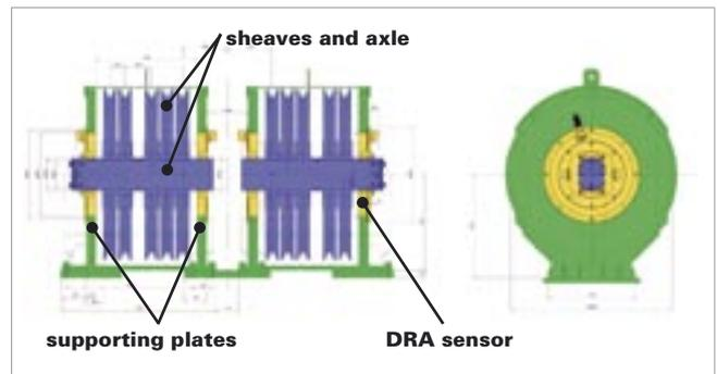
**Fig. 7: Basic structure of an upper sheave block weighing system**
