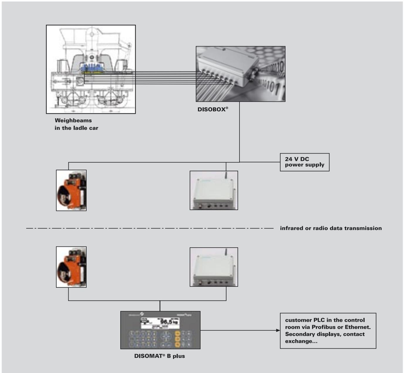
**Figure 19. Application example for a ladle transfer car weighing electronics**
