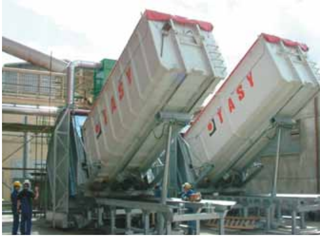
Fig. 5 Docking station with tipped container
