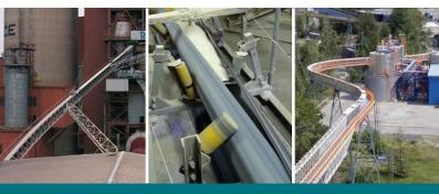
The tube belt conveyor is closed during transport and thus ensures material conveyance with minimal spillage and significantly less contamination in the conveying process. One of the main advantages is the ease of integration into existing plants to ensure flexible and reliable transport. Schenck Process uses TEDO technology to produce customised tube belt conveyor designs.
