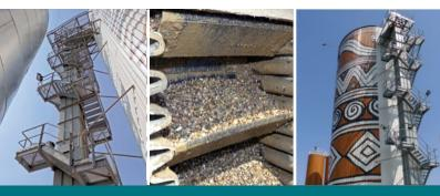
The corrugated belt conveyor is designed for vertical conveyance and requires only minimum maintenance. The system conveys material both horizontally and vertically, using just one transport device. The rigid base belt features vulcanised cleats and flexible corrugated side walls that are suited to transporting a wide range of materials. Inclined or vertical conveyors are always tailor-made turnkey solutions based on state-of-the-art TEDO technology.
