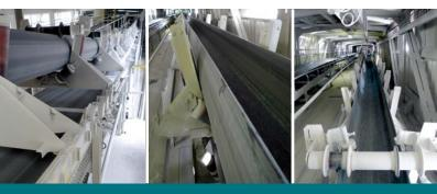
U belt conveyors offer the same advantages as tube belt conveyors when it comes to flexible positioning. However, these conveyors achieve significantly higher feed rates than traditional tube belt conveyors. In other words, a smaller and lighter self-supporting steel structure is used for the same feed rate.
