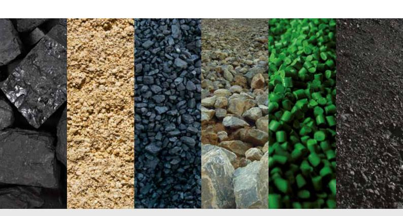
Schenck Process has an extensive materials database covering over 10,000 samples where characteristics such as particle size distribution, shape, porosity, bulk density, temperature, moisture content, fragility and air retentiveness have been measured and the most suitable conveying method determined.
