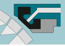
The seal automatically inflates only when the dome is fully closed.
