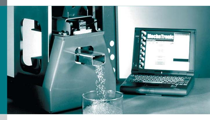
The MULTIGRAV® feed station comprises 1 to 8 system modules designed for continuous gravimetric feeding of granules. An optimised vibro feeder delivers the granules into the process. The system module is connected to a weighing module with optimised centre of gravity. The weighing module incorporates the vibration-resistant load cell.
