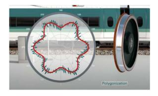
MULTIRAIL<sup>®</sup> Wayside Train Monitoring has a measurement uncertainty of just ± 1 %, even at train speeds of 80 km/h.
