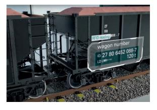
Weighing in accuracy class 0.2 per **OIML** means a permissible tolerance of 200 kg for a 100 t wagon.
