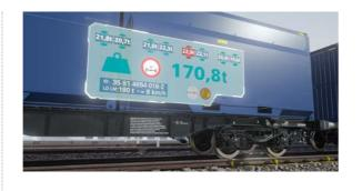
Axle load weighing helps improve the safety of material handling within transport.
