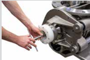
2. Remove shaft guards, outer cover and pull rotor to endplate with rotor removal tool.
