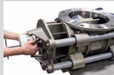
3. Slide out endplate and rotor.
