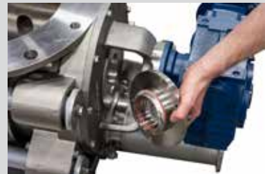
6. When bushing is removed unit is disassembled.
