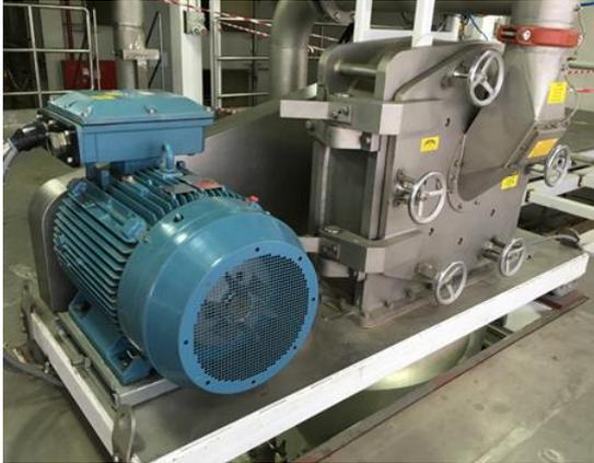
Shown below is a PPS 7CMT mill and the mill's interior, depicting the rotor and classifier, supplied for milling Lactose.
