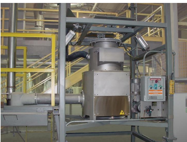
The feeder is connected to a graphical interface and recipe management system that allows an operator to set the feeder parameters and monitor its operation from one central location.
