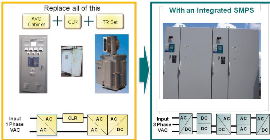
**Fig-1: Conventional Power Supply System vs. ModuPower High Frequency Power System**
