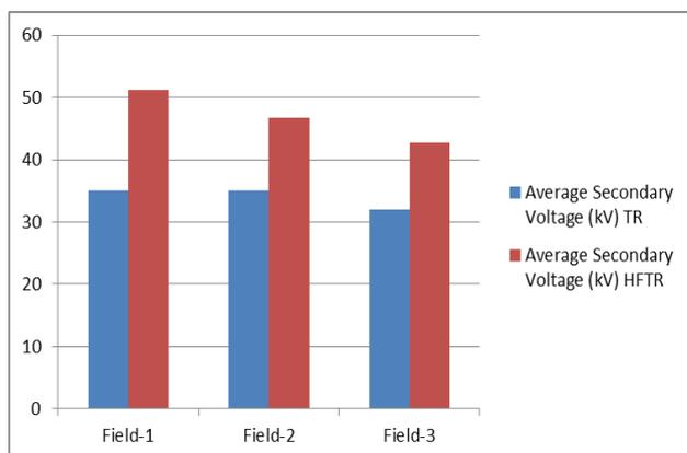
**Figure 5: kV comparison between TR vs HFTR**
