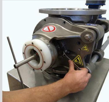
2. Remove shaft guards, outer cover and pull rotor to endplate with rotor removal tool.
