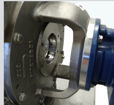
6. When bushing is removed unit is disassembled.
