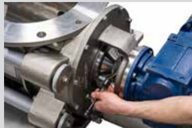
5. Loosen the bolts around the bushing and seal assembly, then remove the bushing and seal assembly.
